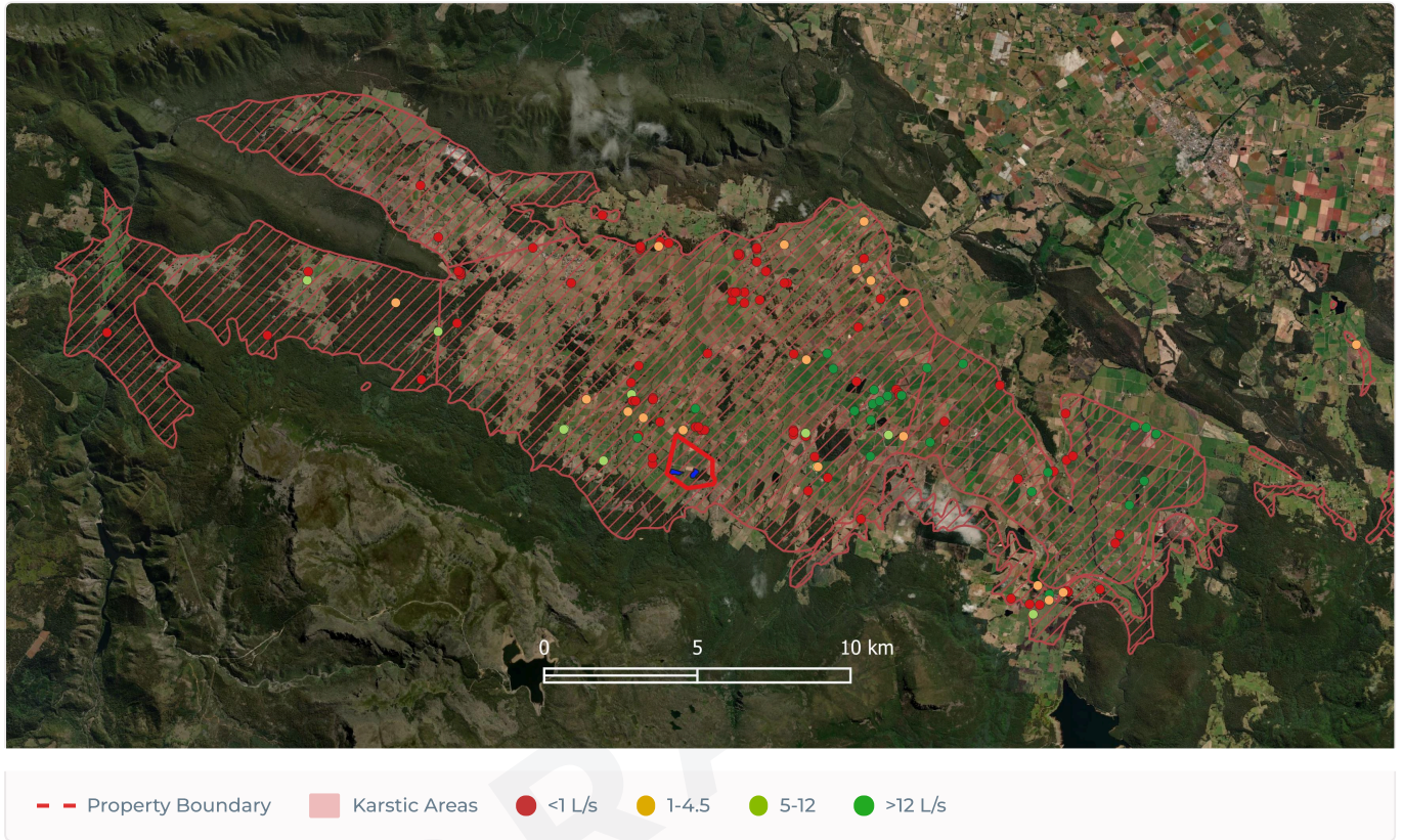
FIGURE 7. REGIONAL BORE YIELD MAP. COLOURED MARKERS INDICATE RECORDED YIELDS FROM HISTORICAL DRILLING.
